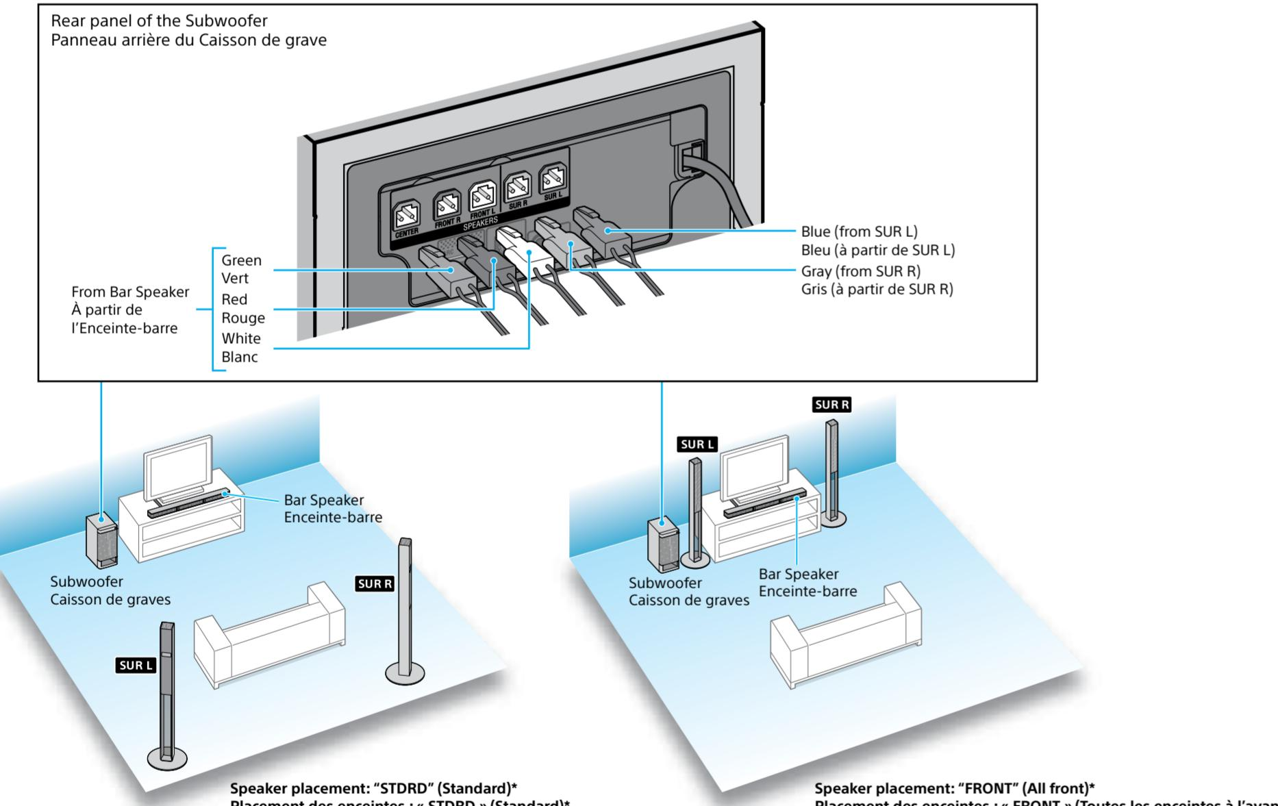
\* To select speaker placement, refer to "Using the setup display" in the supplied Operating Instructions.
