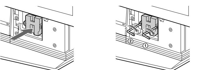
Mount the new lamp securely into the lamp receptacle.
