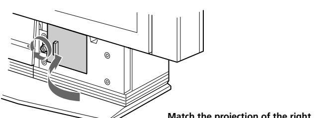
Match the projection of the right side of the lamp cover with the hole of the unit, and replace the lamp cover as it was.
